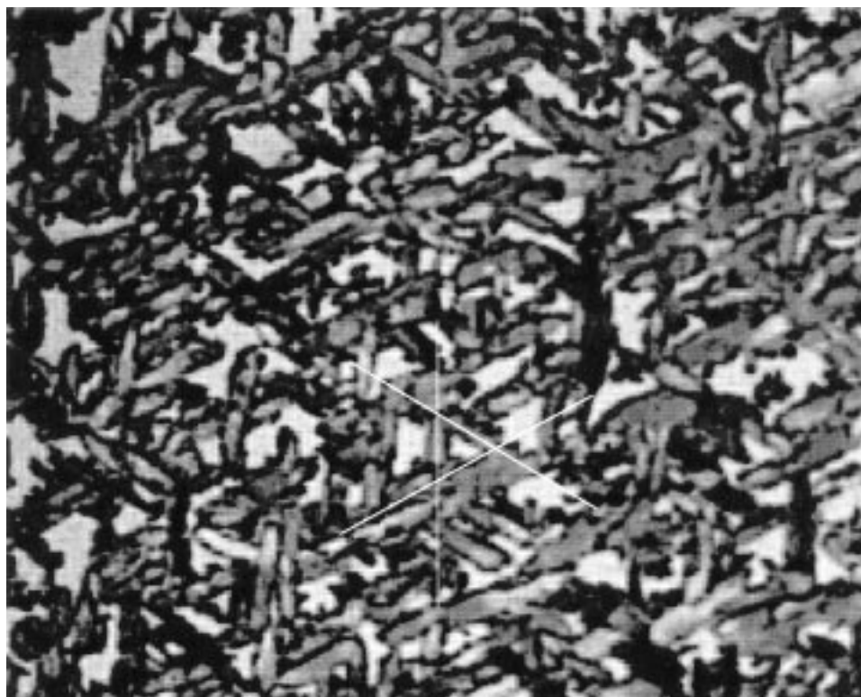
Figure 2. Reflectance polarization light micrograph (approximately 300x magnification) of uracil crystals on the surface of MoS 2 . The three-fold symmetry of the underlying substrate is represented in the adsorbate crystals (indicated by the white lines) and shows heteroepitaxial registration of the adsorbate on the substrate.
