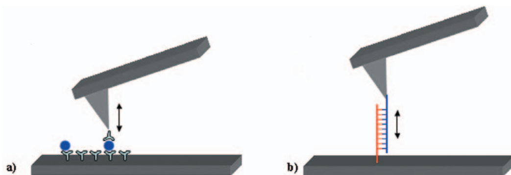
Figure 1. Schematic set up of force spectroscopy experiments: By immobilizing a molecular partner either over AFM tip and substrate AFM can test a) intermolecular interactions between receptor and ligand; and b) complementary nucleic acid binding between DNA strands.
