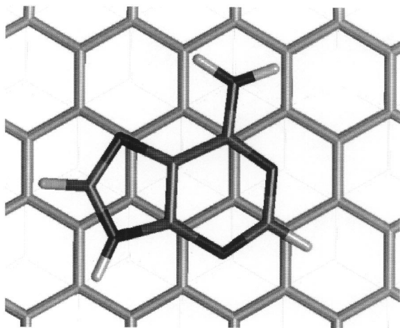
Fig. 3. Top view of the minimized structure of one single adenine molecule on a 3-layer graphite slab. Only the first graphite layer is shown. The molecule lies flat above the graphite surface.
